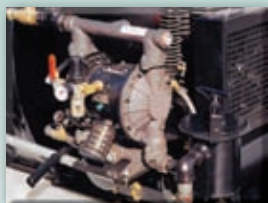
Air Driven Dual Diaphragm Pump with Basket Strainer
