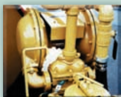
Hydraulically Driven Dual Diaphragm Material Pump
