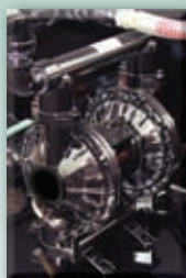
Dual Diaphragm Material Pump
