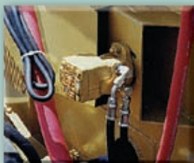
Hydraulically Driven Agitation
