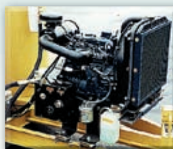
Liquid Cooled 14.5 H.P. Kubota Diesel Engine
