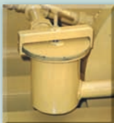
Easy Access Basket Strainer Reduces Tip Clogging
