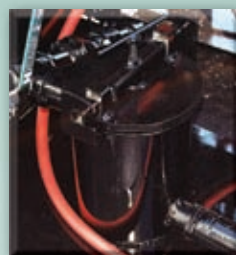
Easy Access Basket Strainer Reduces Tip Clogging
