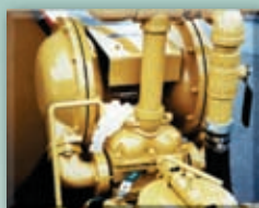
Hydraulically Driven Dual Diaphragm Material Pump
